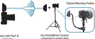
Camera with Plus® III in hot shoe (Transmitting)
